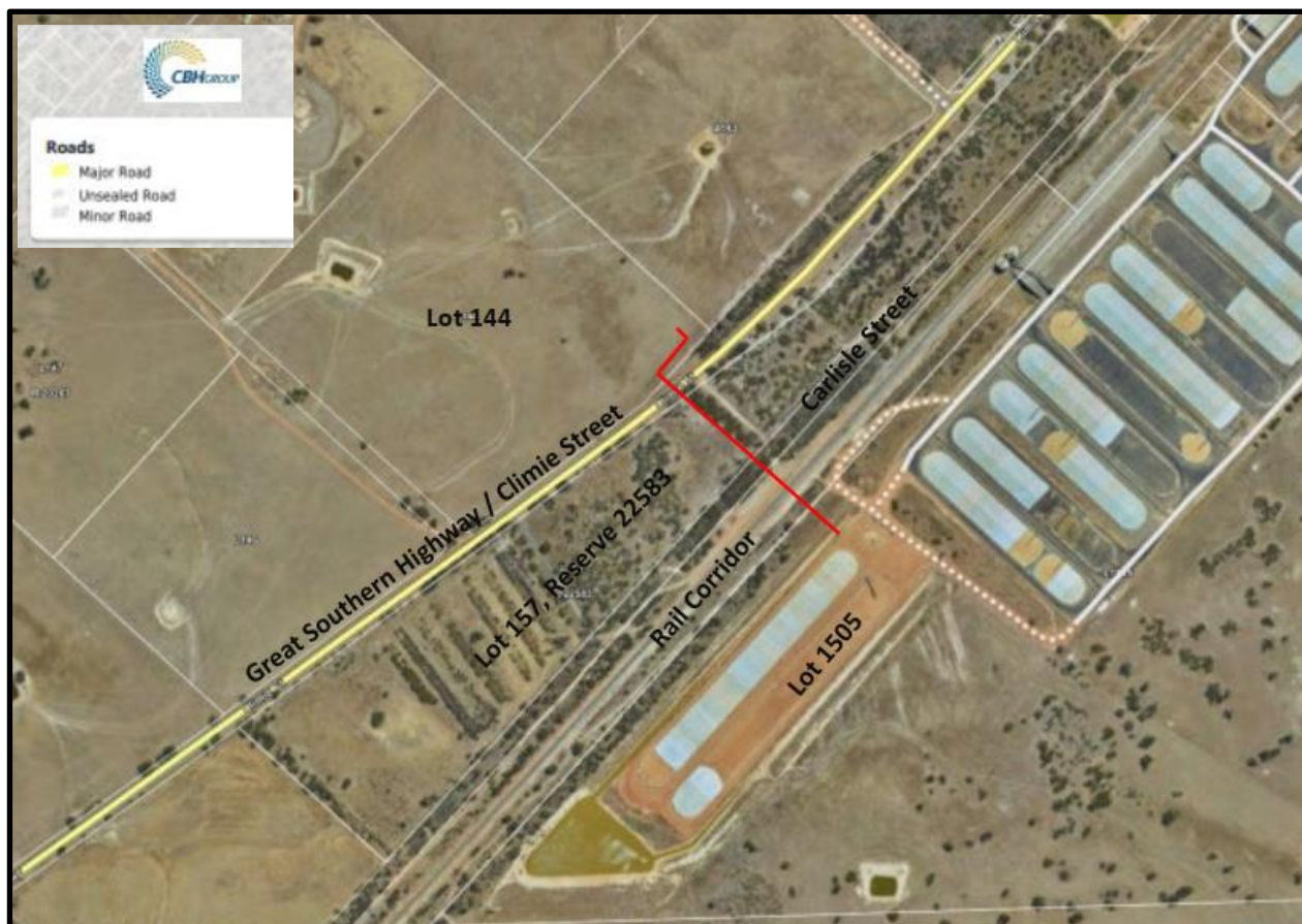
Above: Simplified site plan showing approximate route for underground power in a red line Plan is not to scale
